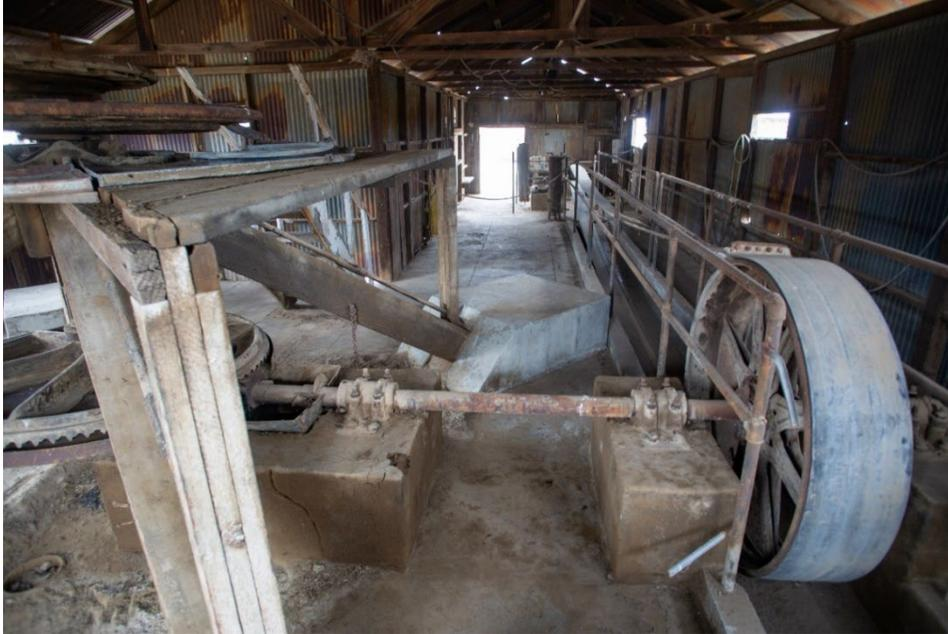
**Photo 18** The 12x12 timber supports above the horizontal ring gear and the vertical drive shaft. The oil pan under the ring gear is visible. The camera is facing south.
