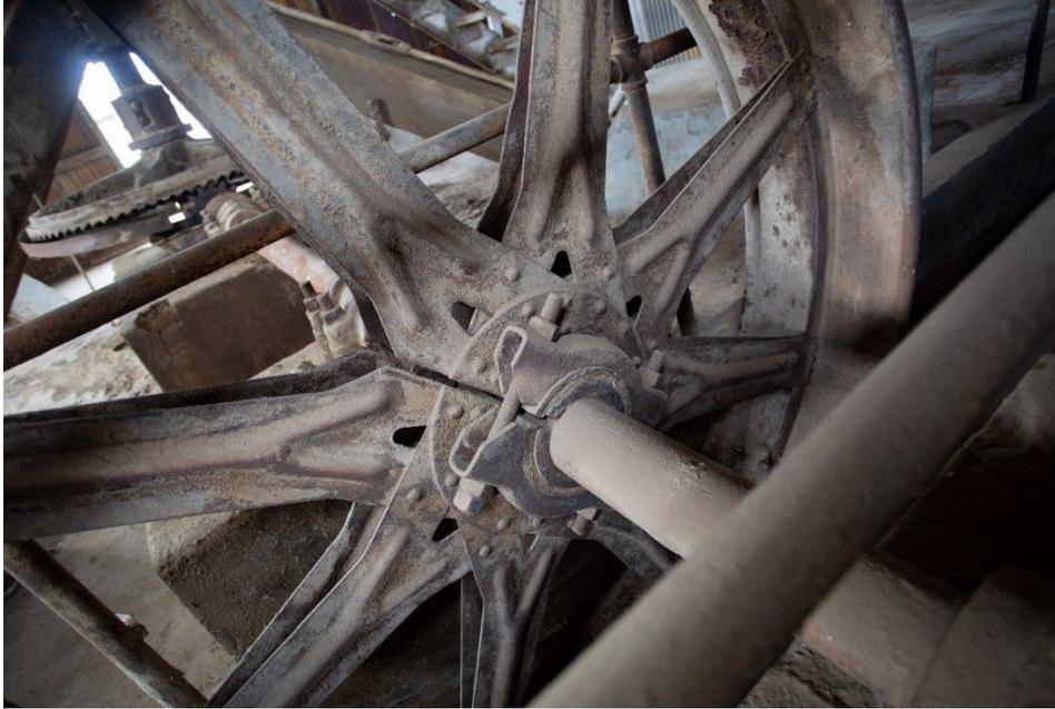
**Photo 16** The drive wheel and the long belt. Also shown is the concrete raceway beneath the belt, and the guards. The camera is facing north.
