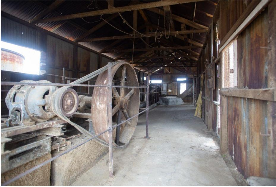
**Photo 14** General view of the building's interior and almost the whole operating system, including a top view of electric motor and v-belts on the drive wheel, the long drive belt on the left of the photo, and machinery at the far end of the Jack Plant. The camera is facing south.
